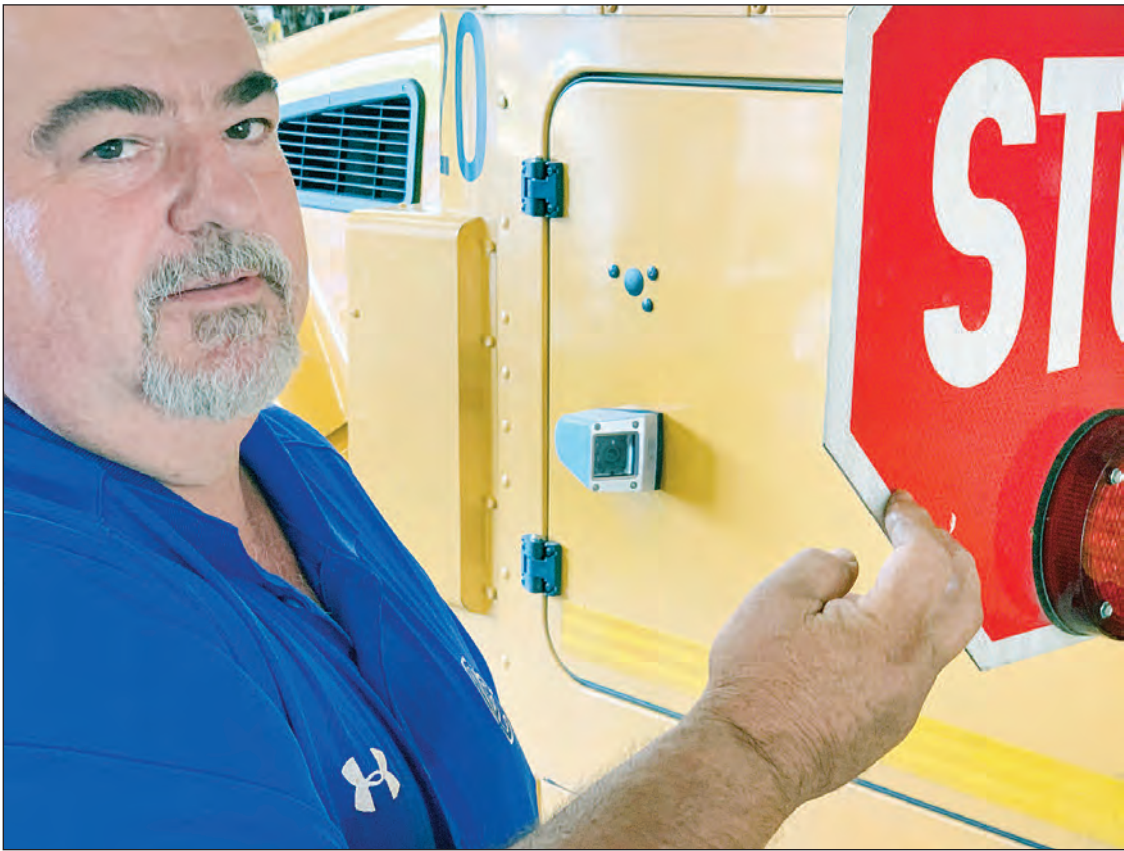
Crittenden County Schools Transportation Director Wayne Winters shows off one of the stop-arm cameras (center of image) installed on district buses to photograph the license plate of a motorist who fails to heed bus warnings. An average of one local incident a day sees a driver run school bus stop arm warnings.
